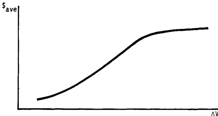
FIGURE 12-3. AVERAGE REPAIR COST VERSUS CRASH SEVERITY
