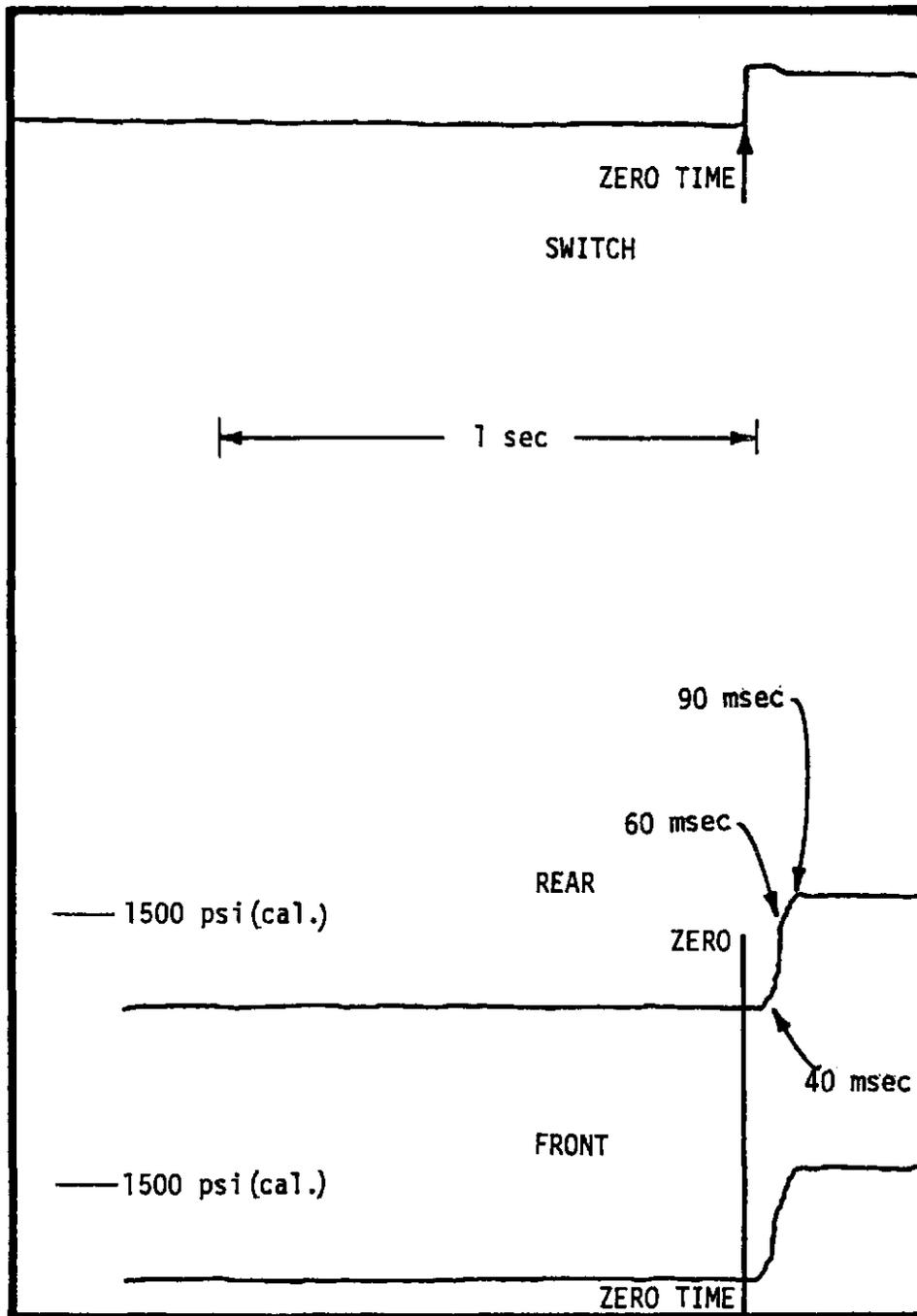
Note: "Zero time" refers to the time at which an electrical signal is sent to the CMS solenoids. The pressures shown here were measured just upstream of the anti-skid brake pressure modulators.
