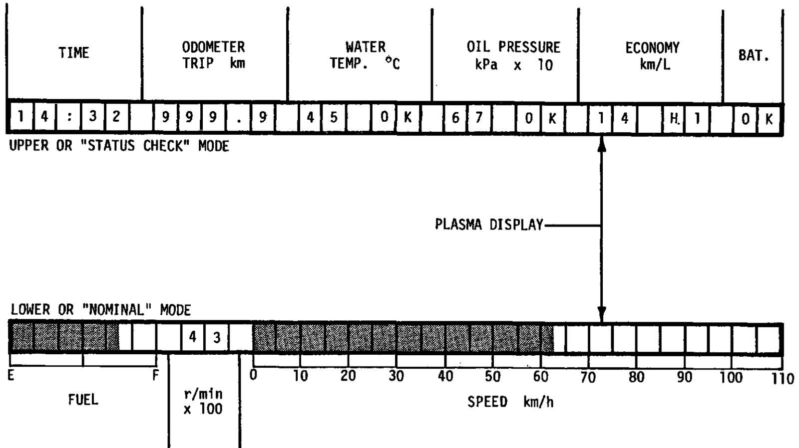
FIGURE 8-2. HIGH TECHNOLOGY DRIVER DISPLAY
