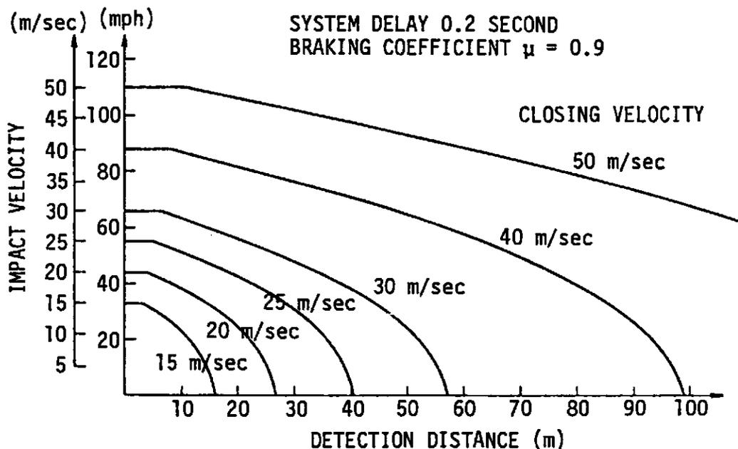
FIGURE 9-9. IMPACT VELOCITY AS FUNCTION OF DISTANCE BETWEEN RADAR CAR AND COLLISION OBJECT
