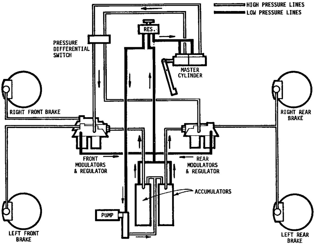
FIGURE 5-6. HYDRAULIC SCHEMATIC OF THE
