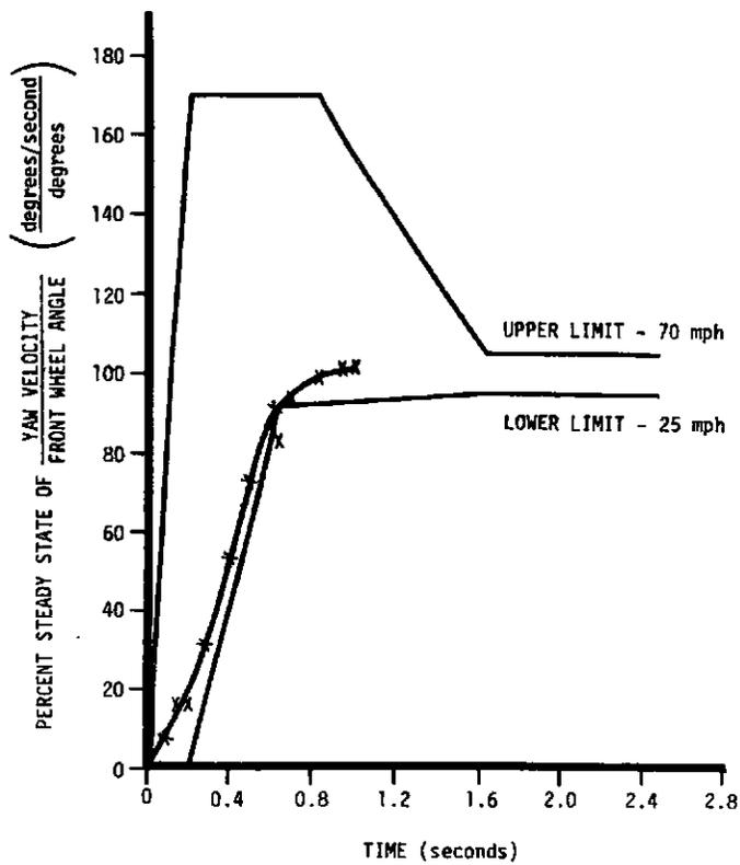
FIGURE 10-3a. TRANSIENT YAW RESPONSE VS. TIME AT 25 MPH CLOCKWISE
