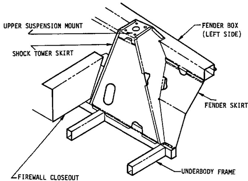
FIGURE 11-4. SUSPENSION MOUNT – FIRST DESIGN ITERATION
