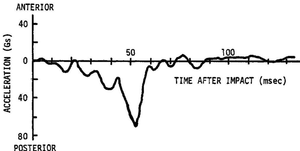
FIGURE 3-2. CHEVROLET VEGA LONGITUDINAL MID-COMPARTMENT ACCELERATION DURING 30 MPH ALIGNED FRONTAL BARRIER IMPACT (MINICARS TEST 1060-2)
