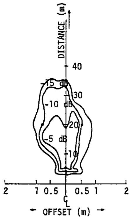
FIGURE 9-5. COVERAGE PATTERN Ku-BAND RADAR - OUTPUT OF POSTAMPLIFIER
