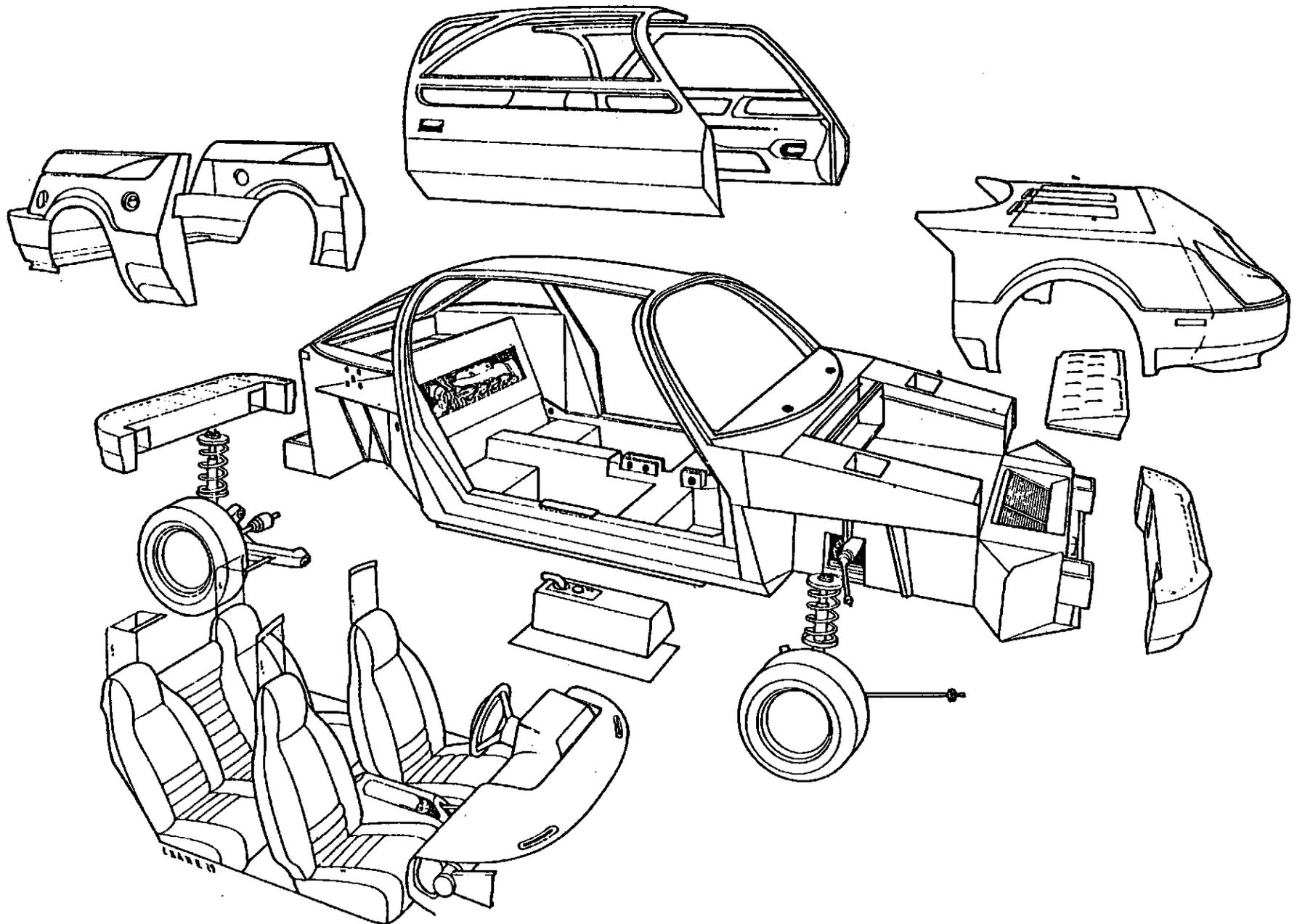
FIGURE 2-1. MAJOR RSV INTERIOR AND EXTERIOR BODY COMPONENTS
