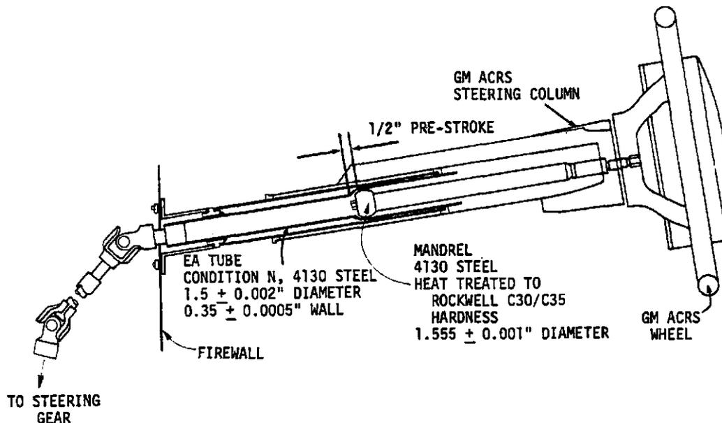
FIGURE 4-9. COLUMN STROKING MECHANISM
