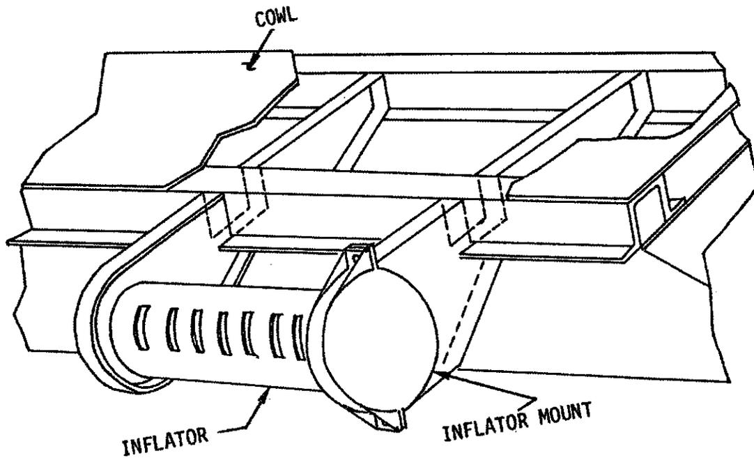
FIGURE 4-15. PASSENGER RESTRAINT BRACKETS
