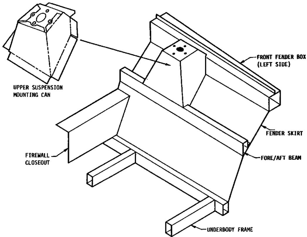
FIGURE 11-5. SUSPENSION MOUNT - SECOND DESIGN ITERATION
