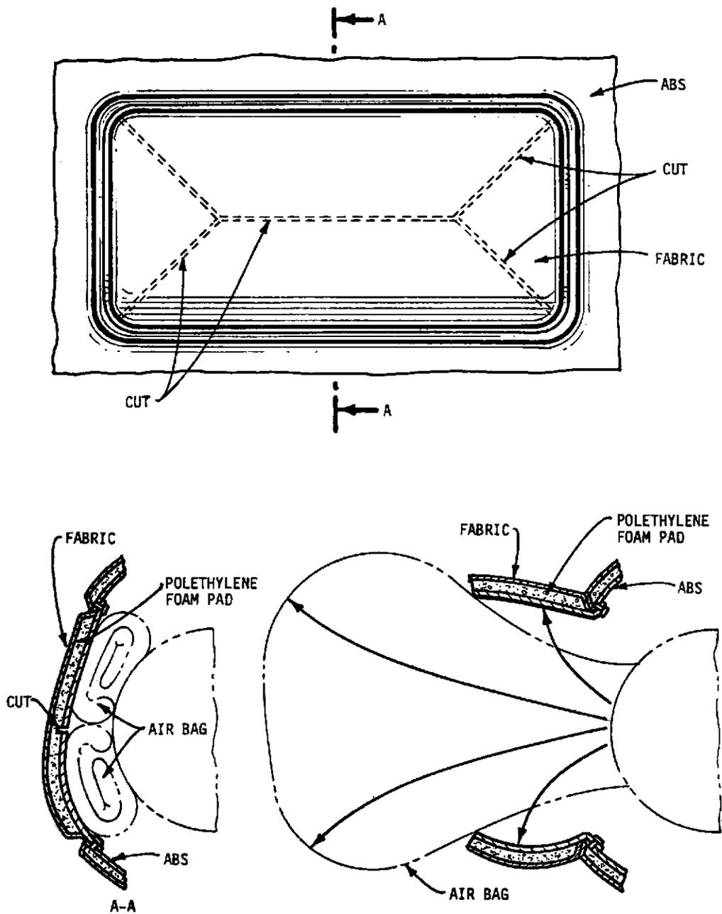
FIGURE 4-17. PASSENGER ACRS COVER AND OPENING SEQUENCE
