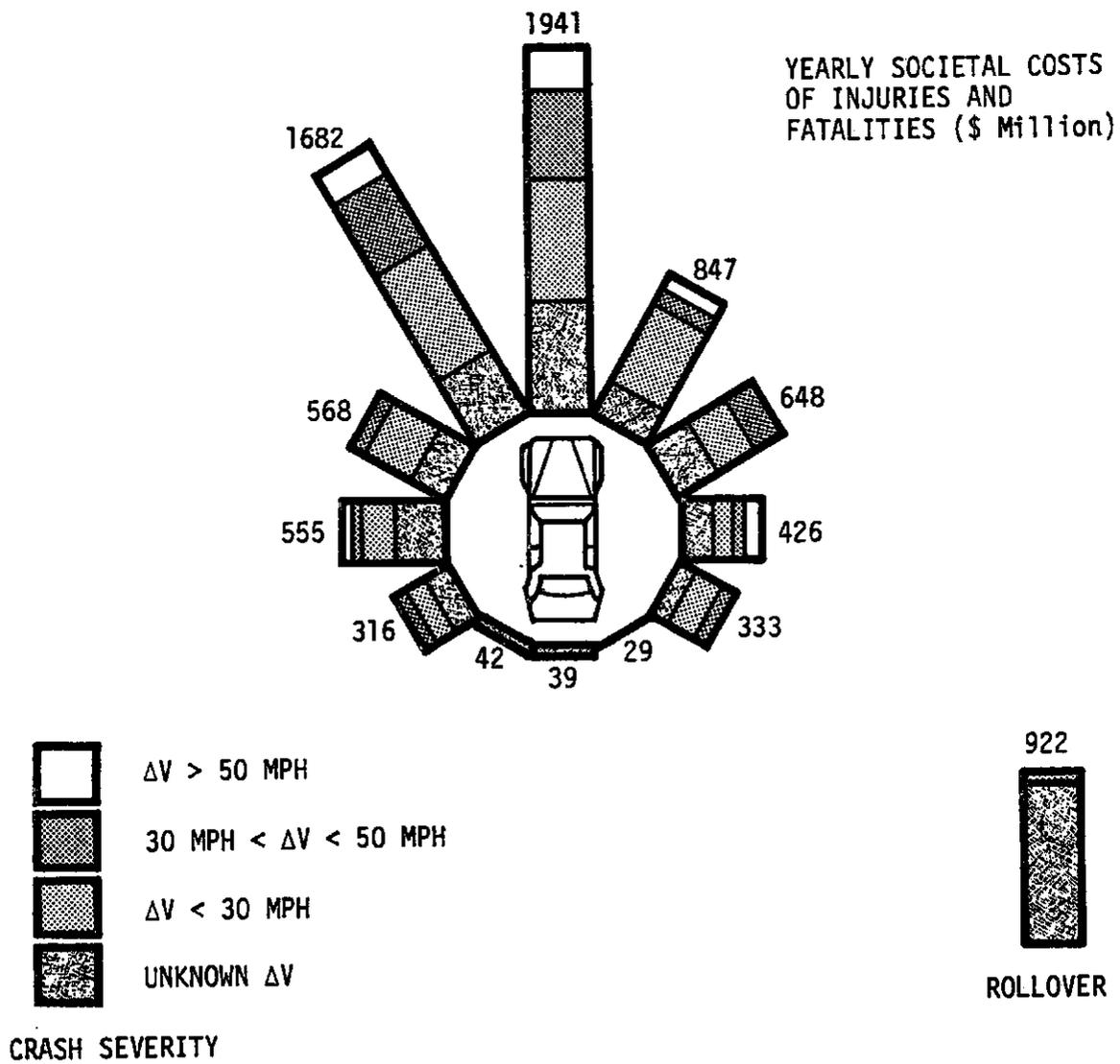
FIGURE 1-2. SOCIETAL LOSSES FOR THE VEHICLE DAMAGE AREAS
