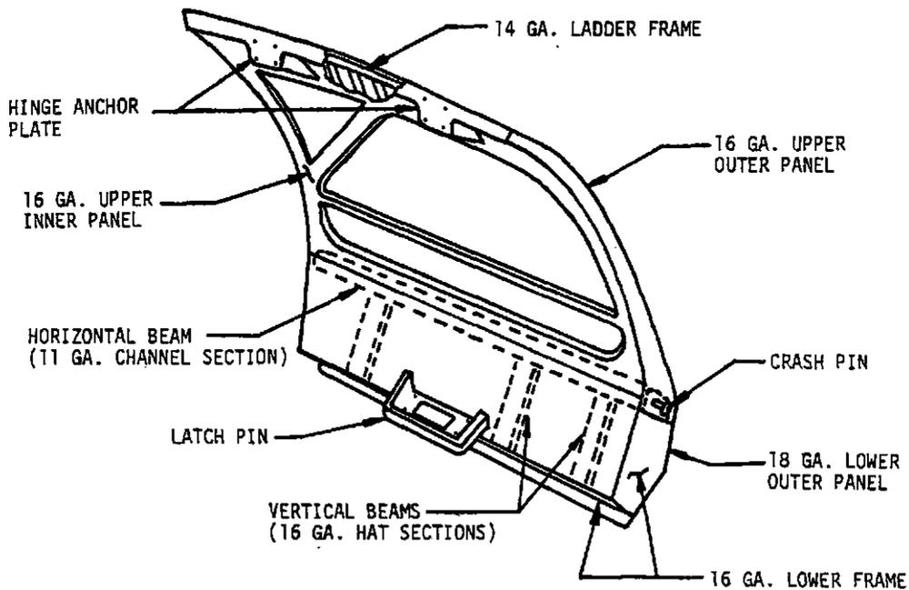
FIGURE 3-6. GULL WING DOOR STRUCTURE
