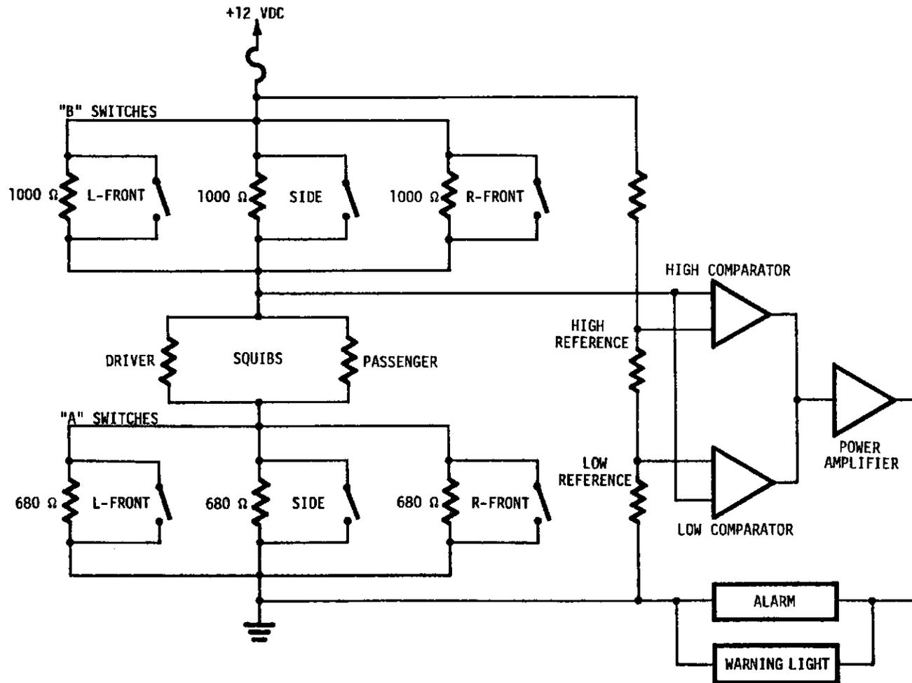
FIGURE 4-13. SIMPLIFIED ACRS CIRCUIT DIAGRAM
