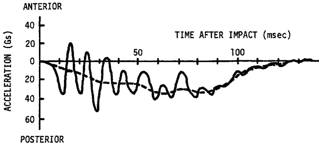
FIGURE 3-5. RSV LEFT REAR COMPARTMENT LONGITUDINAL ACCELERATION DURING 47.6 MPH ALIGNED FRONTAL BARRIER IMPACT
