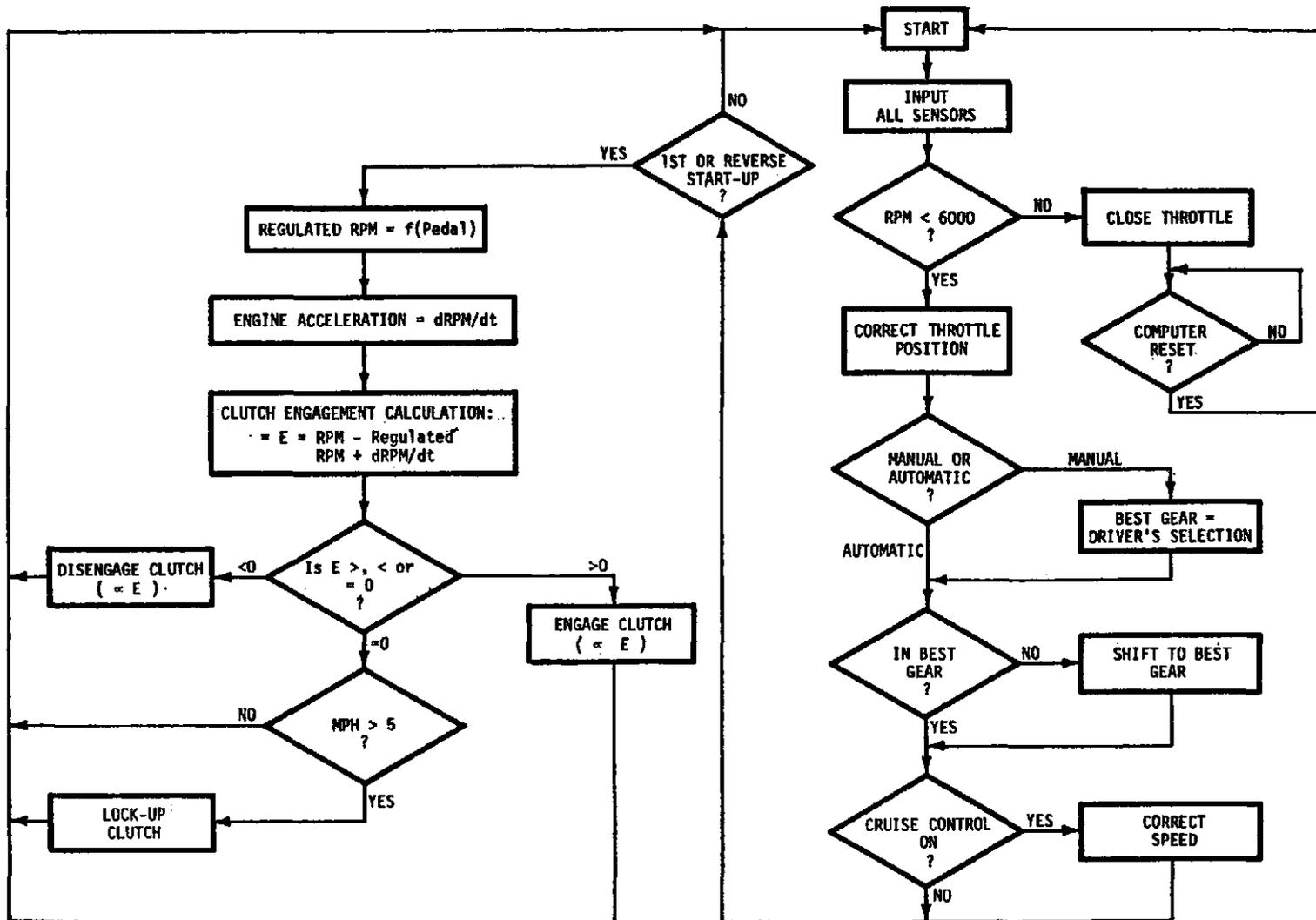
FIGURE 6-2. FLOW DIAGRAM OF THE AUTOMATED MANUAL TRANSMISSION
