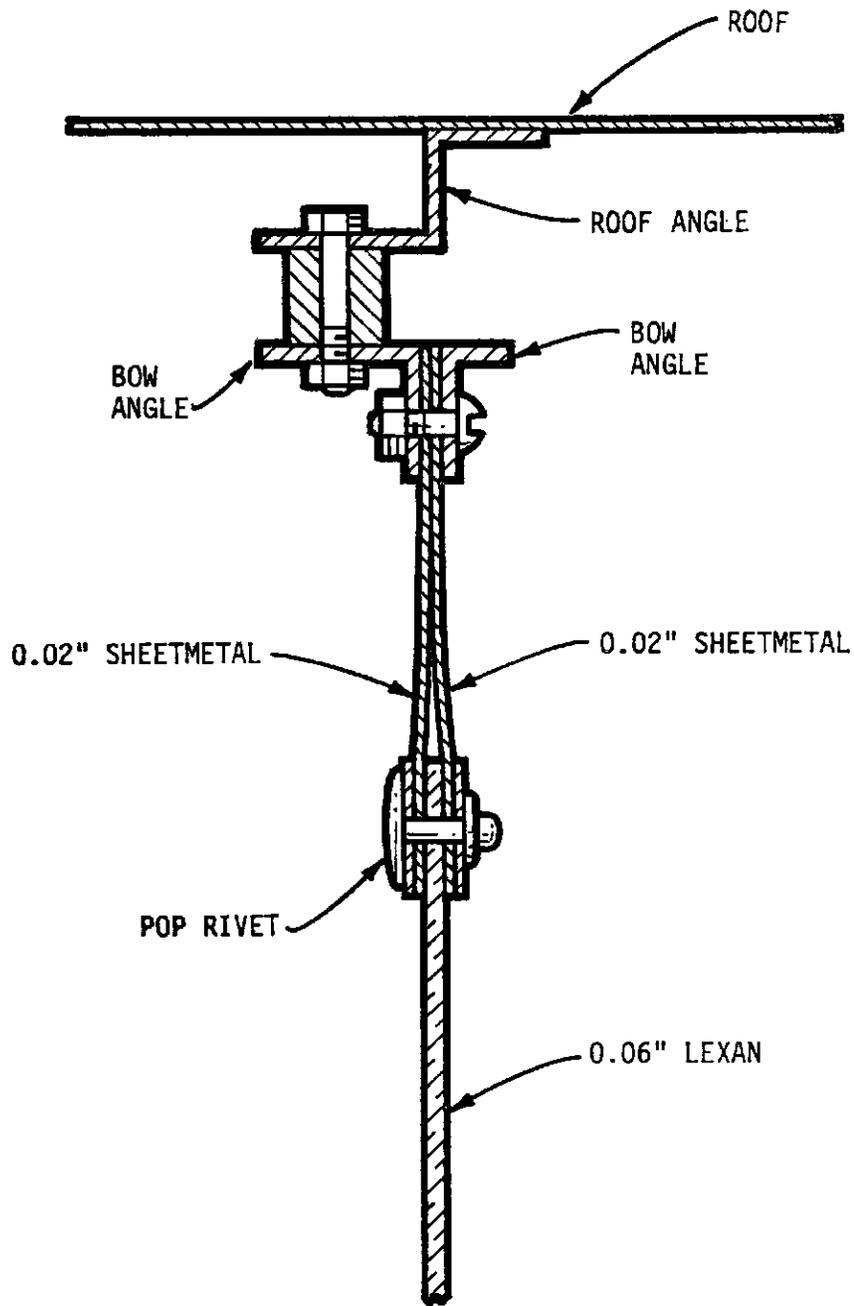
FIGURE 4-21. FRONT SEAT/ROOF ATTACHMENT ASSEMBLY
