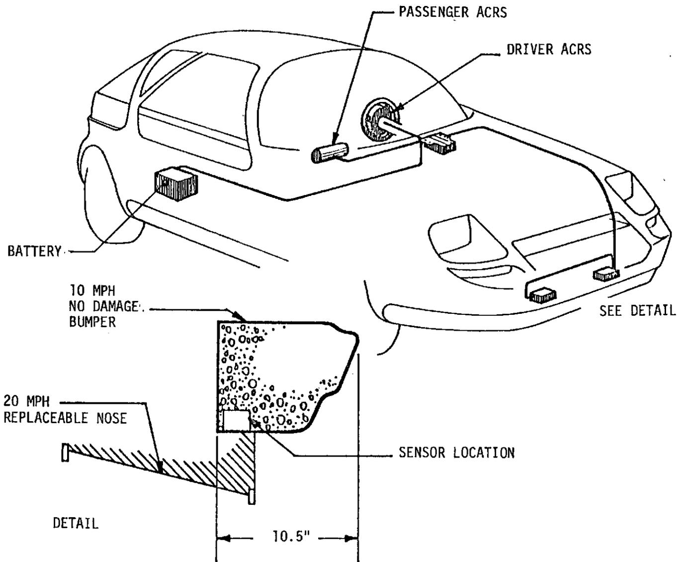
FIGURE 4-4. PHASE II SENSOR SYSTEM
