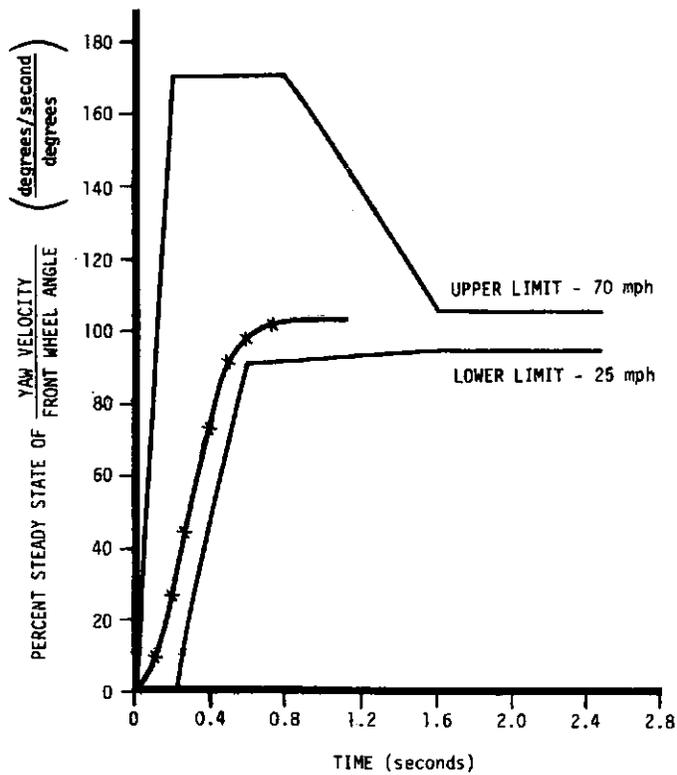
FIGURE 10-3b. TRANSIENT YAW RESPONSE VS. TIME AT 25 MPH COUNTERCLOCKWISE
