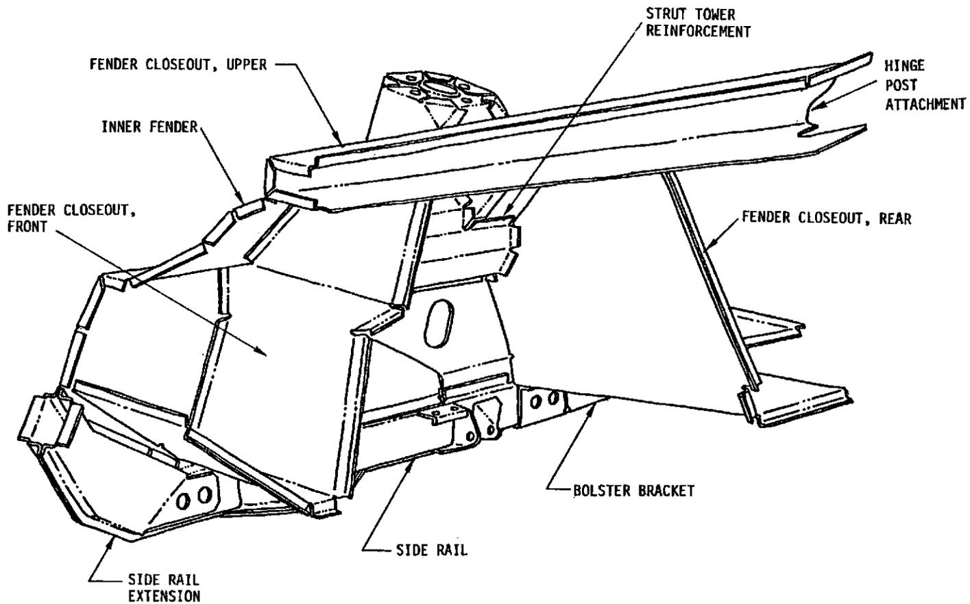
FIGURE 11-13. LEFT FRONT INNER FENDER WELDMENT
