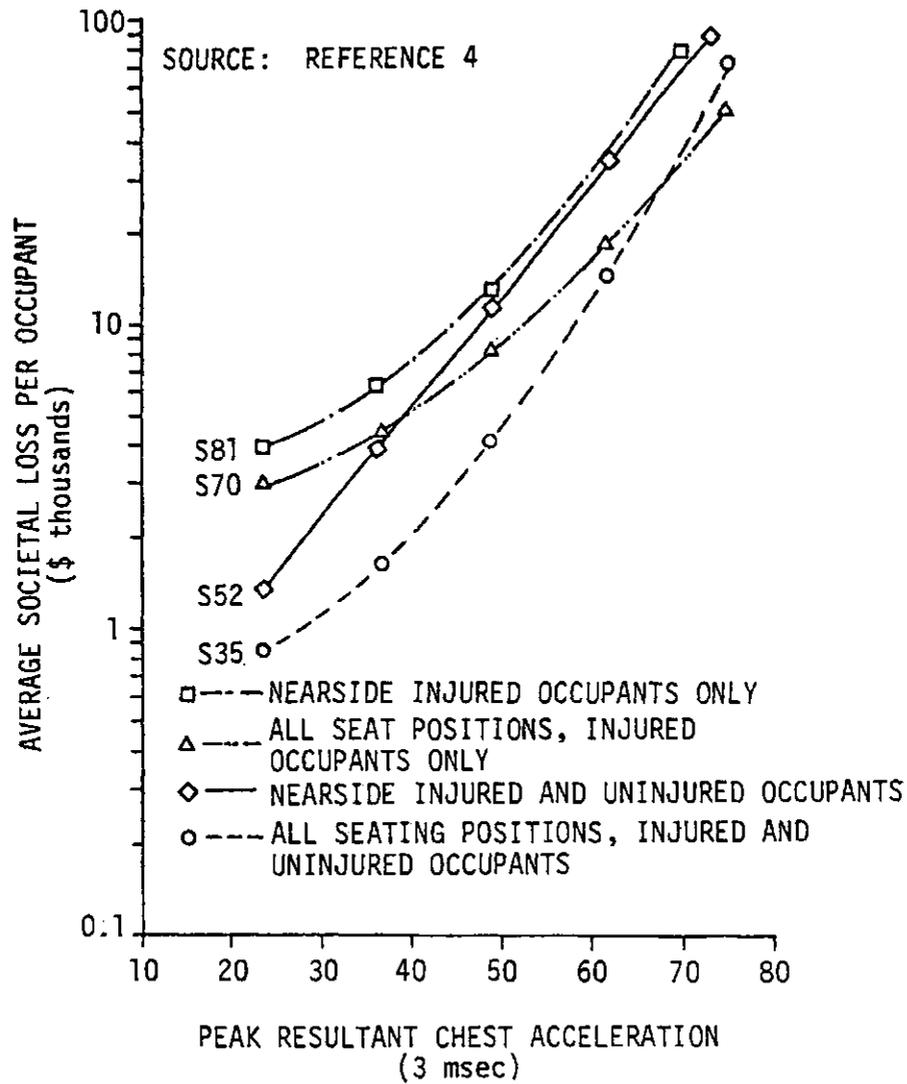
FIGURE 3-8. INJURY MEASURE-TO-SOCIETAL COST TRANSFORMATIONS, WITH CRUSH AS A PARAMETER
