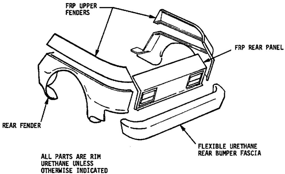
FIGURE 7-2. REAR EXTERIOR PARTS
