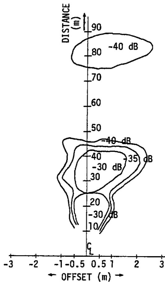
FIGURE 9-4. COVERAGE PATTERN Ku-BAND RADAR - OUTPUT OF PREAMPLIFIER
