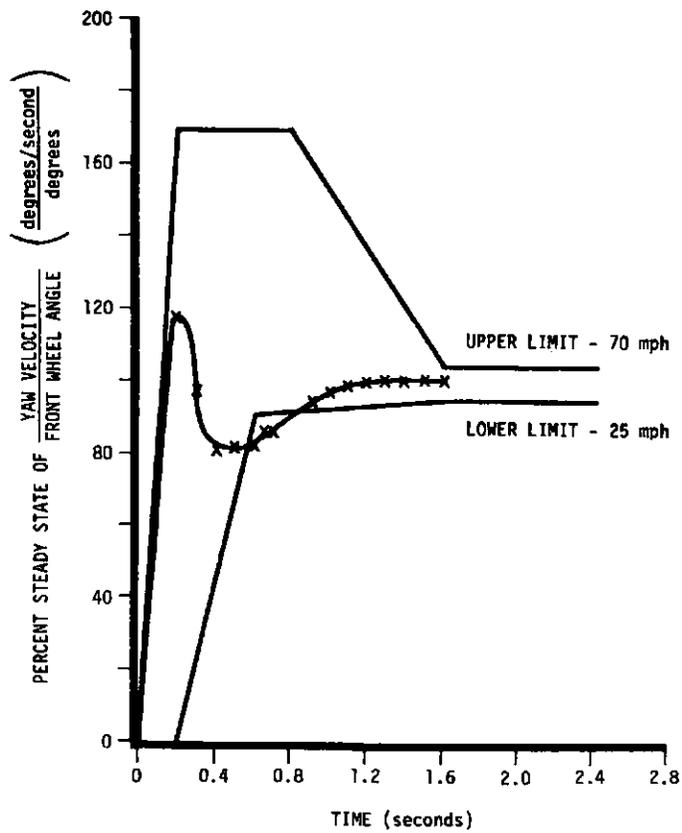
FIGURE 10-3c. TRANSIENT YAW RESPONSE VS. TIME AT 50 MPH CLOCKWISE
