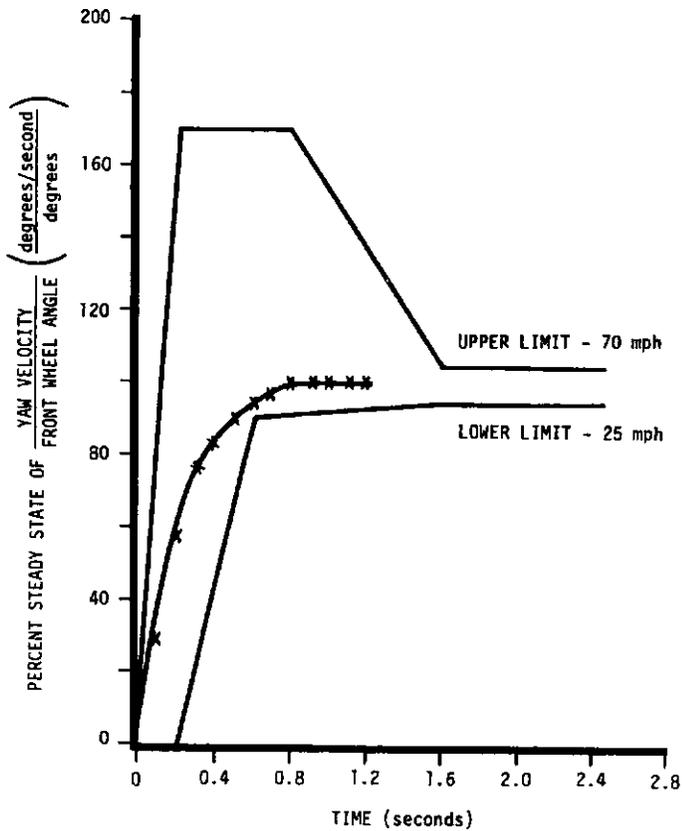
FIGURE 10-3d. TRANSIENT YAW RESPONSE VS. TIME AT 50 MPH COUNTERCLOCKWISE
