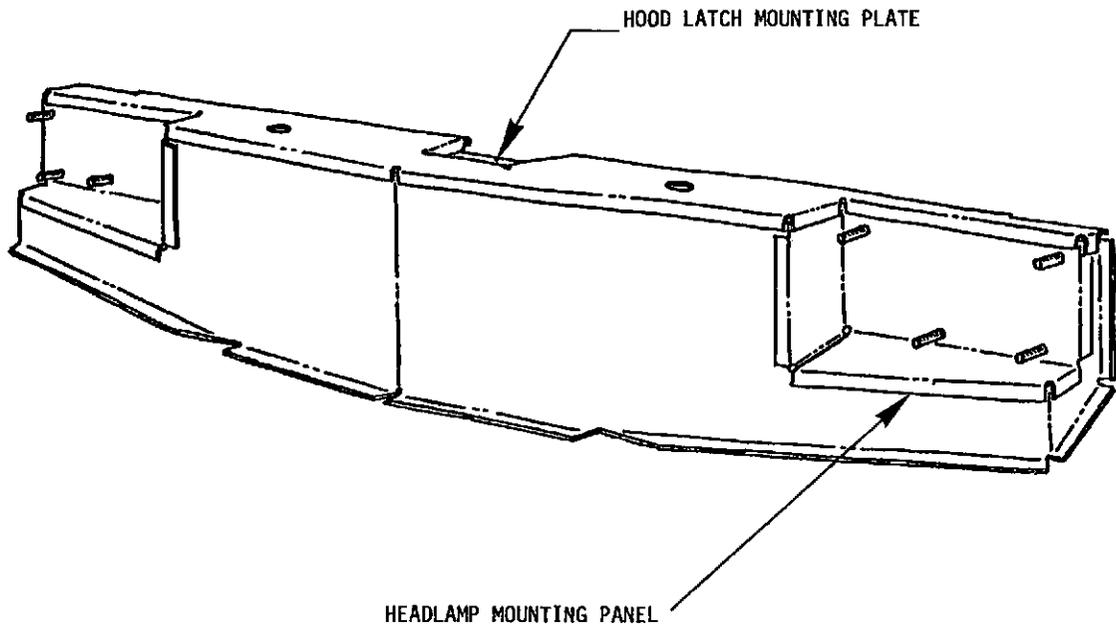
FIGURE 11-11. FRONT IMPACT BEAM WELDMENT
