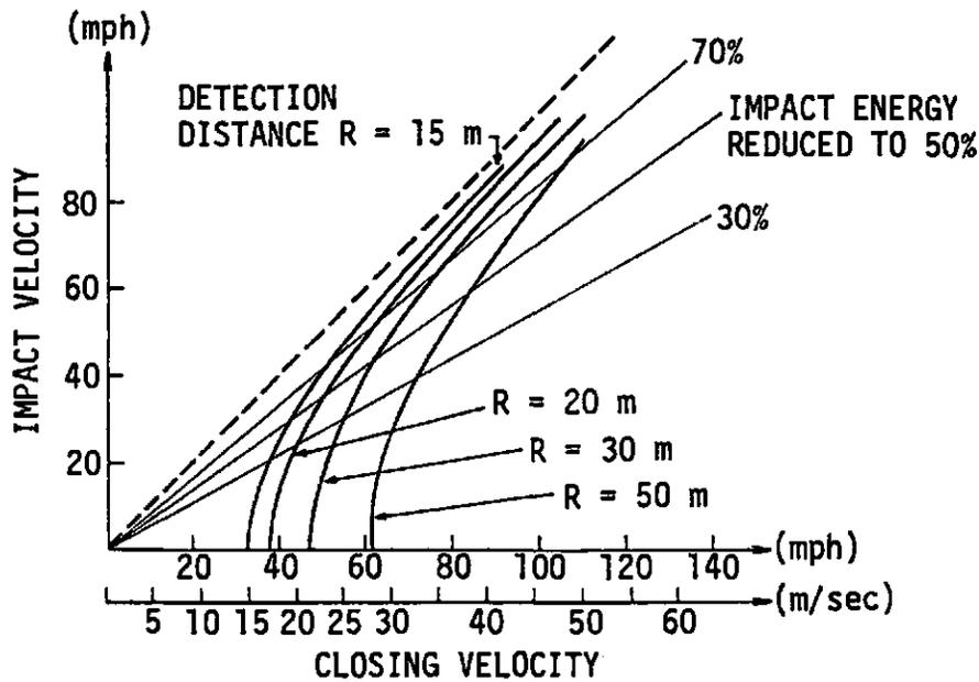
FIGURE 9-10. ENERGY REDUCTION AS FUNCTION OF DETECTION DISTANCE AND CLOSING RATE
