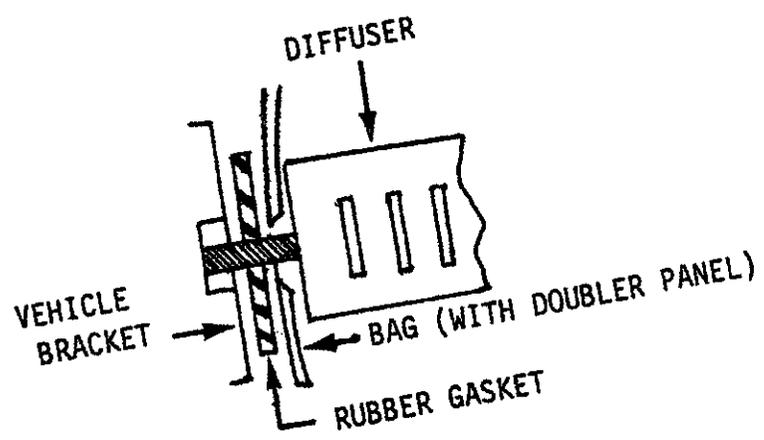
FIGURE 4-16. AIRBAG CLAMPING CONFIGURATION
