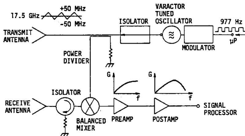
FIGURE 9-2. Ku-BAND FMCW RADAR
