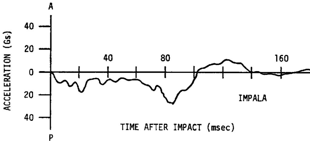
FIGURE 4-24. LONGITUDINAL MIDCOMPARTMENT ACCELERATIONS IN 78.5 MPH RSV/IMPALA ALIGNED FRONT IMPACT
