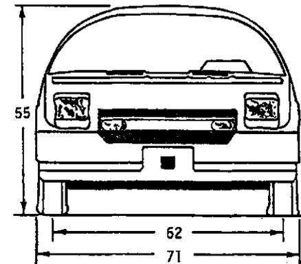
FIGURE 8-3. SIGNIFICANT RSV DIMENSIONS (IN INCHES)
